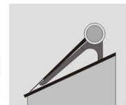
Sloping roof installation
