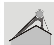
Sloping roof installation
